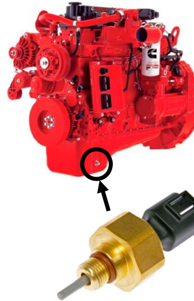
Figure 7. Cummins Diesel Engine showing oil sensor location and current design (left) and thermocouple sensor used in design (right)
