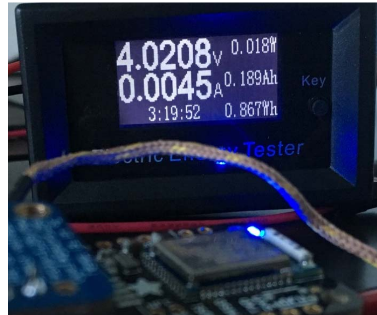
Figure 15. Power Monitor tool showing battery voltage, current draw, and power consumption of wireless sensor during operation.
